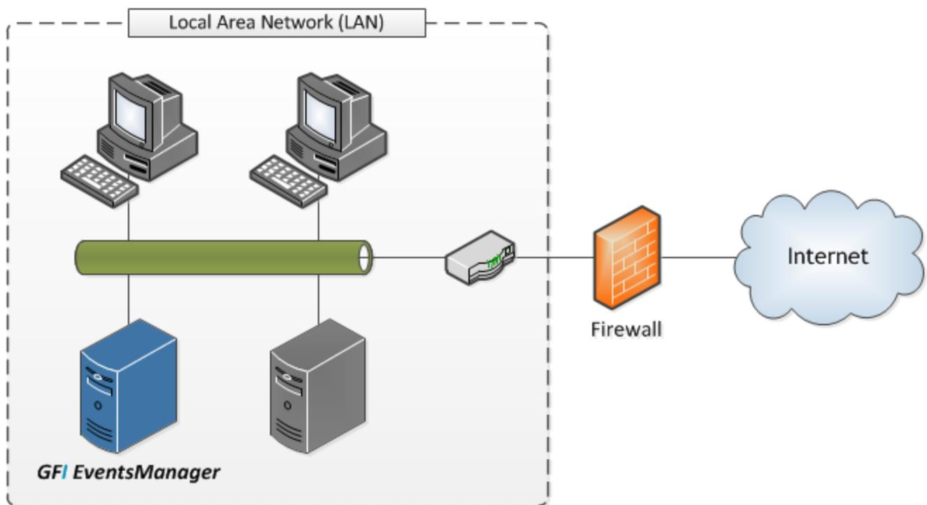
Figure 2: Deployment of GFI EventsManager in LAN
