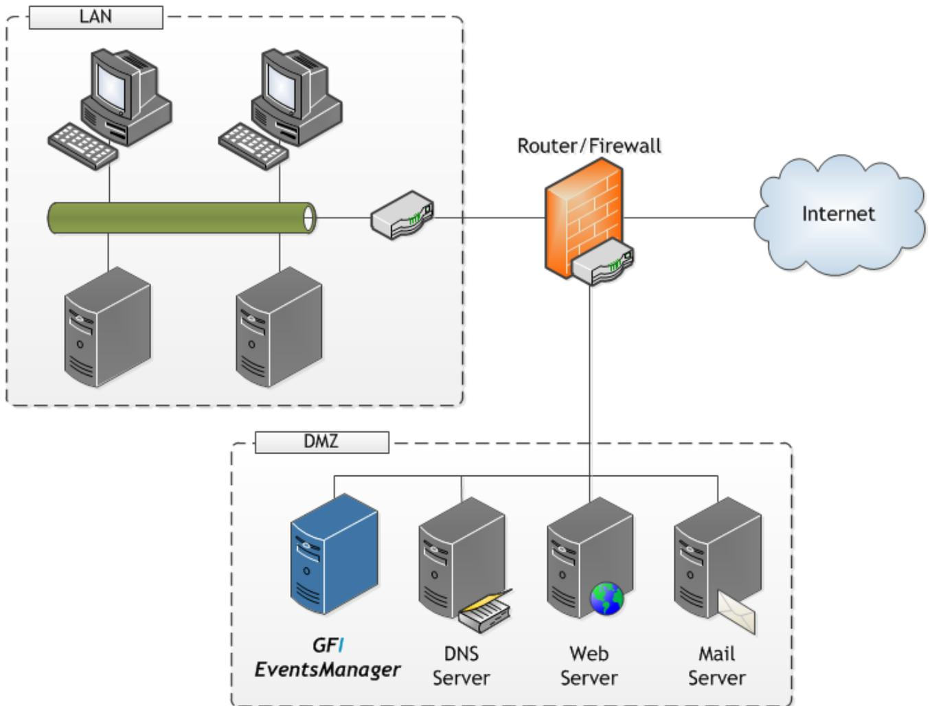
Figure 3: The DMZ sits between the internal LAN and the Internet
